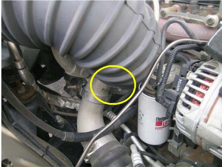
2. Using the pliers, remove the crimp style clamp from the hose on the brass fitting located on the now exposed lower front side of the turbocharger. Remove the hose from the brass fitting and dispose of the crimp style clamp.
