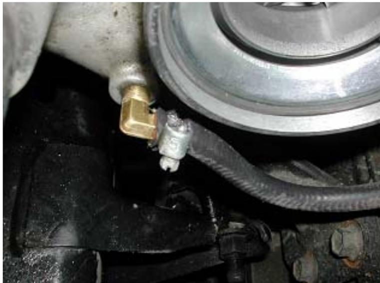
**Note:** *On 2001 auto's turbos, the wastegate is a solid line and does not have a brass elbow to be replaced*
