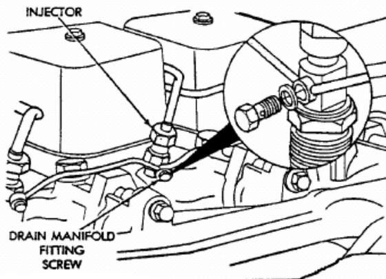
**Fig 13: Fuel Drain Manifold Fittings - Typical**
