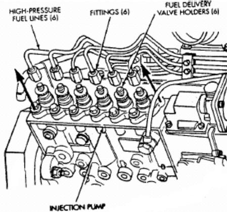
*Fig 11: Delivery Valve Holders and Pressure Lines*
