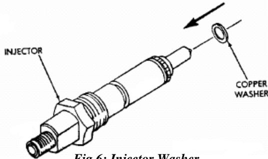
*Fig 6: Injector Washer*
