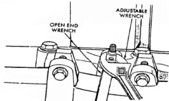
**Fig 3: Loosening injector**
