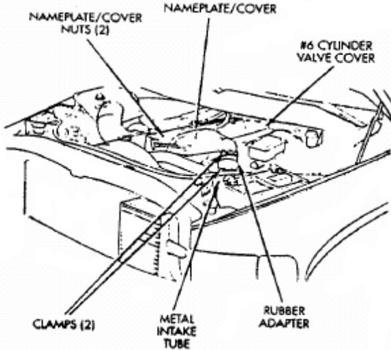
*Fig 9: Nameplate/Cover - Diesel*
