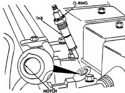
*Fig 8: Installing Injector*
