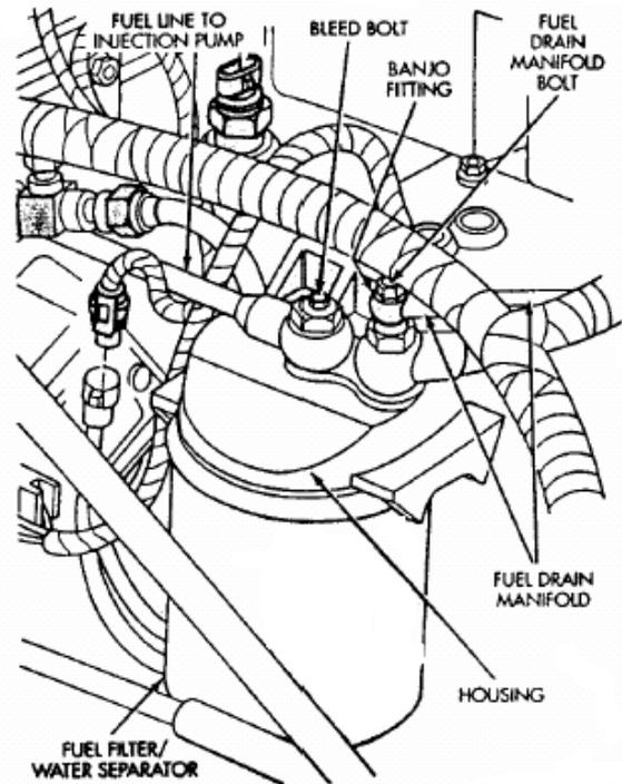
**Fig 14: Drain Manifold and Fuel Filter/Water Separator**
